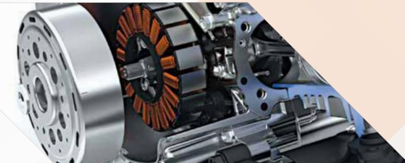
Grazia is equipped with ACG starter, which starts the engine silently by removing gear meshing noise. It also reduces maintenance.
